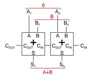
to make a *N*-bit adder, just *daisy chain N* single-bit full adders together
