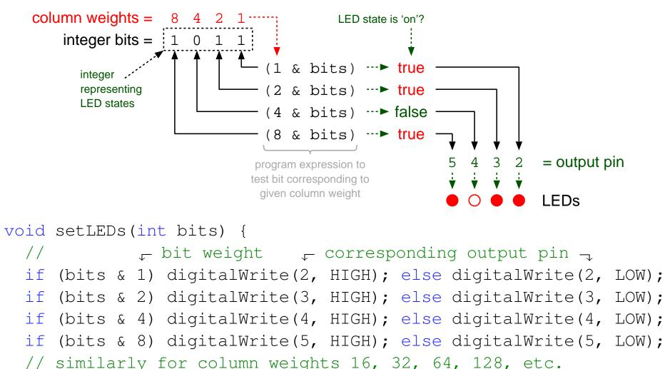
e.g:  $12_{10} = 1100_2$  represents pins 5 and 4 being HIGH, and pins 3 and 2 being LOW
