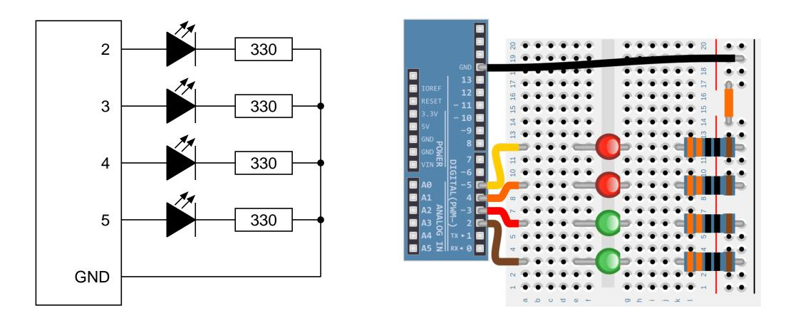
connect up to 20 LEDs (or other digital devices)
