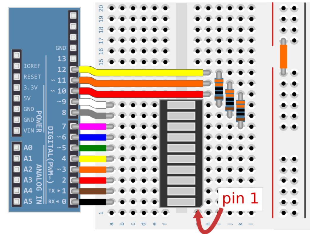
pins 0 to 9 drive anodes of each segment
